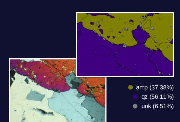
Plane-polarized and cross-polarized images are imported into the software; grain boundaries are identified and mineral phases classified through cutting-edge machine learning algorithms.
